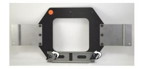
Loosen the 2 knobs and place the bill of the hat under the bill clamp.
