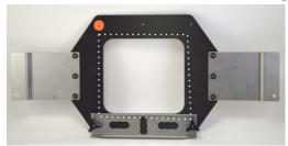
Cut a piece of adhesive backing large enough to cover the sewing field. Place the backing on the underside of the frame sticky side up.
