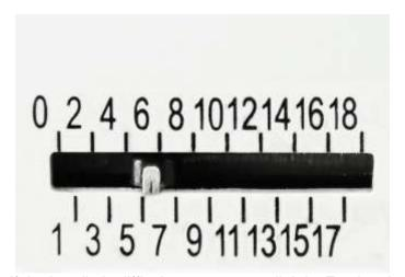
If the handle turns too easily, tighten slightly; if the handle is difficult to turn, open slightly. Forcing the handle causes the handle to spring back if turned too hard. Open up the rollers with a small turn to find the correct setting.
