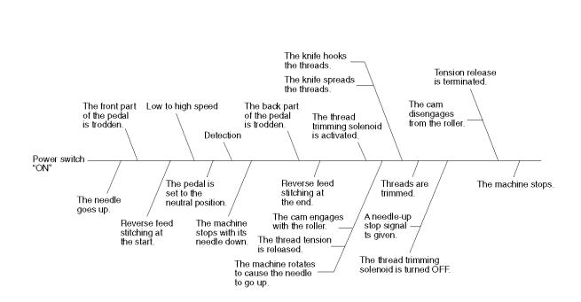
(Caution) The above chart assumes that the switches for automatic reverse feed stitching at the start and end have been set to "ON".
