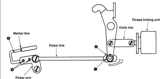
Positioning the thread take-up picker **3**: When the thread take-up pickers touched the bobbin, adjust so that the end of the thread take-up picker **3** is aligned with the right end of the marker line.
