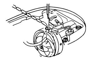
3) The moving knife hooks the needle and bobbin threads (advances).
