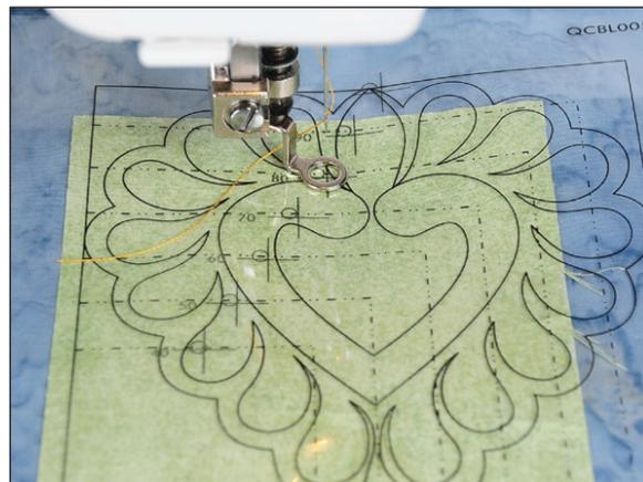
Once you have fine tuned the carriage to the correct position, pull up your bobbin thread and press 'GO'. QBOT will begin sewing the design at the correct scaling percentage.
