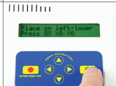
This method is a short-cut in operating the QBOT. Whenever you keep the position of the right-upper and left-lower corners at the same point, QBOT knows that you want to scale to 100% and the position of the sewing machine is the lower-left corner of the design.
