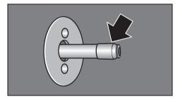
A connecting piece between the brew unit and the main dispenser is located on the inside of the door.
