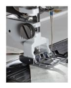
able – when not in use, simply store it in one of the ample accessory trays. Adding and removing is easy! AcuFeed™ now comes in two useful options. The two-pronged AcuFeed™ feet advance fabric flawlessly from the top and bottom. Use this system for quilting, seaming, and traditional sewing. Our special one-pronged AcuFeed™ feet give precise control for more detailed work, like installing zippers and matching seams.
