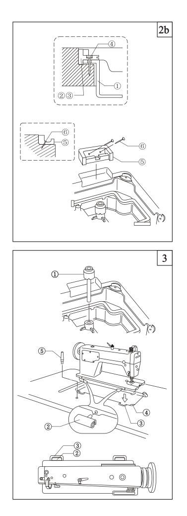
(2) Put the oil pan 1 into the cutouts of table and fix it by nails 4;
