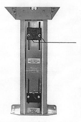
Loosen both 8mm nuts to adjust height of machine to approximately 1/8" above insert level. Tighten nuts.
