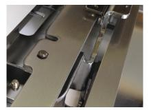
Step 3 - Install the driver assembly as you normally would, tightening the lower (2) thumb screws underneath and the top right side thumb screw, leaving out the top left thumb screw.
