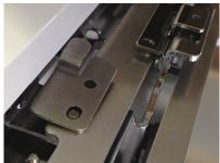
Step 5 - Put the remaining gray plastic thumb screw through the hole in the override bracket and tighten. Make sure that all of the thumb screws are tight and you are ready to sew with your new "Dream Frame"
