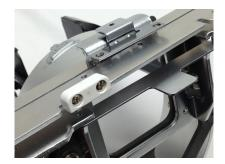
Step 1 - Locate the white plastic magnet cover on the back of the driver assembly. It is on the top aluminum bracket that attaches to the drive bar with (2) gray plastic thumb screws.
