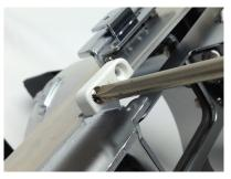
Step 2 - With a Phillips head screw driver, remove the (2) screws and then the white plastic magnet cover. Be careful not to lose the magnet that is inside the plastic cover. Save all the parts for re-installation later.
