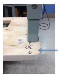
Left side - set the table top bottom side up on a work bench or any convenient work station – from the edge of the table to the to the leg measure 3  $\frac{1}{4}$ " as shown - use the 1  $\frac{1}{4}$ " X 5/16" self tapping screw to anchor the leg.
