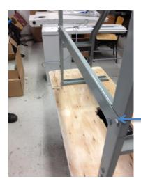
Attach the back brace use (4)  $\sqrt[3]{4}$  X  $\sqrt[3]{8}$  bolt and (4)  $\sqrt[3]{8}$  spring washer (place the spring washer on the inside)
