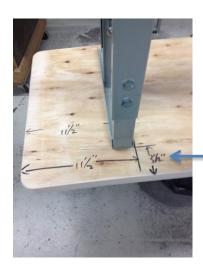
Right side - from the edge of the table to inner side of the leg measure 11  $\frac{1}{2}$ " and 3  $\frac{1}{4}$ " from back edge of the table as shown here – use the 1  $\frac{1}{4}$ " X 5/16" self tapping screw to anchor the leg.
