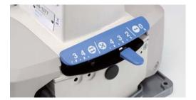
Stitch shape can easily be changed over between (3) and (3) button-hole configurations only by operating the lever.
