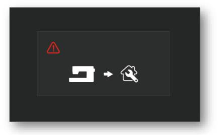
By pressing the "Cancel" button, the user will be reminded when machine is restarted. By pressing the "Confirm" button, the message will no longer be displayed until the next 4'000'000 stitches have been reached. An icon will still be displayed in the software version page until it is reset by a technician after maintenance has been done.
