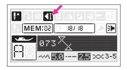
Press the reverse button to cancel the repeat sewing, machine will sew 3 locking stitches at the end of one complete combination. The LCD screen will display the auto-stop icon during sewing the last stitch.
