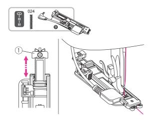
Using the electronic buttonhole foot.
