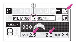
The stitch length, stitch width, mirror and elongation of the stitches can be adjusted manually depending on each stitch settings.
