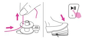
6. Hold the thread tail securely in one hand. Step on the foot control or press the start/ stop button to start winding the bobbin.
