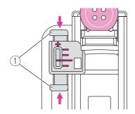
Consider the unique shape of each button, the electronic buttonhole foot allows to adjust the length and width to fit each button. The buttonhole fine tuning adjuster provides a precise setting for buttonhole, and the buttonhole adjustment button (Page 26) allows to adjust the buttonhole size from Small to Large.
