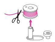
8. Cut the thread and then remove the bobbin.
