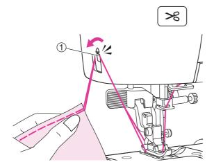
9. Press the thread cutter button to trim the threads.
