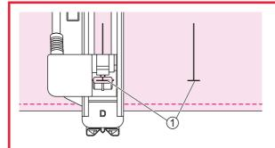
Position the fabric under the presser foot so that the centerline's mark is aligning with the center of the buttonhole foot.
