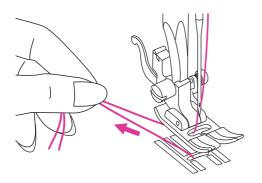
Pull both threads to the back under the presser foot.
