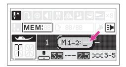
A sub-screen appears. Select a number 1 or 2 of the memory module in the cursor flashing.
