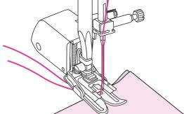
Draw the bobbin thread up and place both bobbin thread and needle thread behind the walking foot attachment.
