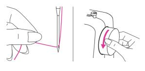
Hold the upper thread with your left hand. Turn the handwheel towards you (counter-clockwise) to lower the needle down below the needle plate then raise it to bring the bobbin thread up.
