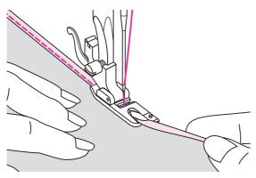
Lower the presser foot lifter and start sewing slowly guiding the raw edge of the fabric in front of the hemmer foot evenly into the scroll of the foot.
