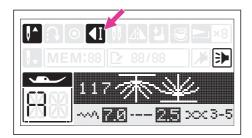
During machine is sewing: When Direct Pattern Group number 6-9 or Regular Pattern Group number 001-009 or 027-128 is selected, the machine will sew 3 locking stitches at the end of the current stitch if the auto-lock button pressed. Then it will stop automatically. The function can be cancelled if pressed the button once again during sewing.
