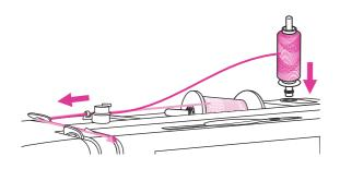
Follow the instructions for single-needle threading using the horizontal spool pin. Thread through the left needle.
