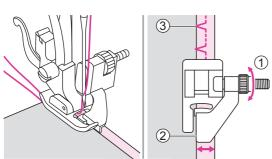
Place the fabric under the foot. Turn the handwheel forwards until the needle swings fully to the left. It should just pierce the fold of the fabric. If it does not, adjust the stitch width accordingly. Adjust the guide by turning the knob so that the guide just rests against the fold.
