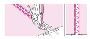
Align the center of the presser foot with the center of the two pieces of fabric and begin sewing.
