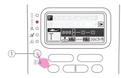
The LED light will be set at Direct Pattern Group. By pressing the pattern group switch button, LED light will move step by step to select the stitch mode.
