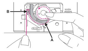
Pull the thread at the arrow markings into the stitch plate thread guide from (B) to (C).
