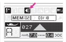
During machine is sewing, the machine will sew 3 locking stitches at the end of the current stitch if the auto-lock button pressed. Then it will stop automatically. The LCD screen will display the auto-lock icon. If pressing the start/stop button again, it will sew from the next stitch.
