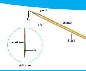
**Point and Tip:** Length, shape and size vary according to needle types.
