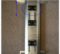
Adjust Plastic Holder move up / down by using Screwdriver
