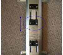
Adjust Plastic Holder move up / down by using Screwdriver
