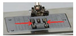
With a short stitch length, the steps are very short. For example when sewing buttonholes and satin stitches. The fabric is fed slowly under the presser foot, even when sewing at maximal speed.
