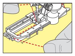
> Pull the cord on the left side under the buttonhole foot to the front.
