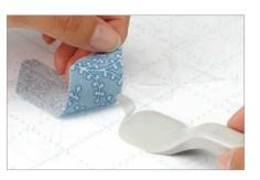
Do not remove the sheet excess. If an uneven surface is created, the fabric may not be cut cleanly.
