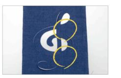
In order to cut cleanly, a mat with an adequate adhesive strength as well as appropriate blade scale and cut pressure settings are required. Replace the standard mat with a new one, and adjust the settings.
