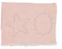
Adjust the Cut Pressure setting and do a test cut.
