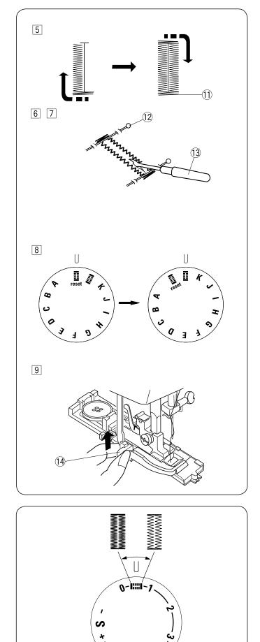
5 Depress the foot control to sew a buttonhole. The machine automatically sews the front bartack, the left row, the rear bartack and the right row. Stop the machine at the ending point.
