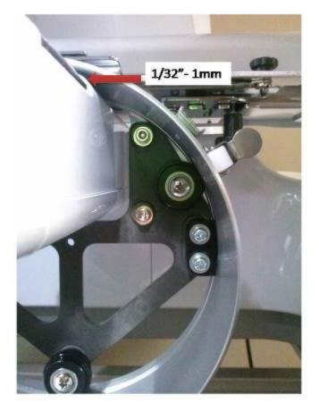
Move/position the black driver ring support down so that the gap between the inside of the aluminum ring is close to but not rubbing on top of the sewing arm. The gap at the corners should be no more than 1/32" or about 1mm. Snug the screws down and check the gap again. Adjust if necessary to maintain the gap, then tighten the screws. With the machine controls, move the driver left and right, front and back to check the alignment. Re adjust if necessary.
