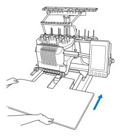
5 While looking below the table, lightly lift it up, and then lower it so that the screw fits into the notch at the front of the guide plate.
