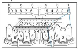
Pass the thread of a specified color through the holes on the thread guide, making sure that you have the thread color matched to the coordinating needle bar.
