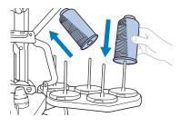
**3** Tie the end of the thread on the new spool with the end of the thread remaining from the previous color.
