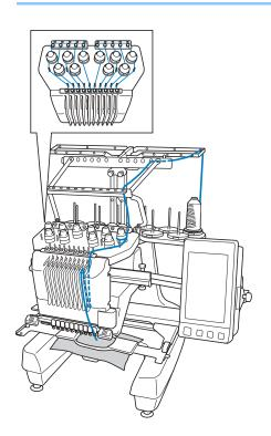
On the spool pin, place a spool with the thread color specified for the corresponding needle bar.
