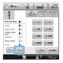
Each time this key is touched, the next color in the thread color sequence display is selected. After reaching the last color in the thread color sequence display, the first color is selected.
