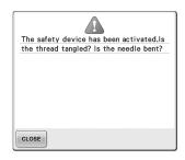
The combined character pattern is The motor has locked up due to tangled thread or for other reasons related to thread delivery. If the thread is entangled in the bobbin case, clean the race, and then oil it. (Refer to page 284 and
