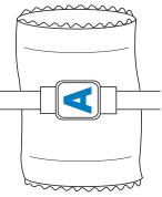
**Example:** When embroidering a T-shirt Rotate the pattern 180 degrees. Pass the machine bed through from the waist of the T-shirt, not from the neck, and attach the embroidery frame to the machine. This will prevent the neck of the shirt from being stretched when the embroidery frame is moving.
