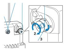
Pass the end of the thread through the guide slit in the bobbin winder seat, and pull the thread. The cutter will cut the thread.
