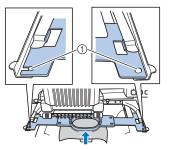
Make sure that the pins on the left and right arms of the embroidery frame holder fit into the positioning slot and hole on the embroidery frame.
