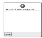
The needle has stopped at an incorrect position. Turn the handwheel so that the mark on the handwheel is at the
