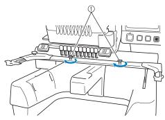
Use the thumb screws included with the machine (thumb screws removed in step 1 on page 261).
