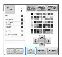
🕨 The 🔊 mark appears to indicate where the machine will stop.
