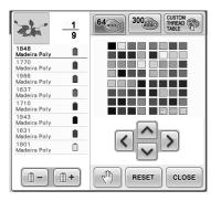
Thread color display using a custom thread
