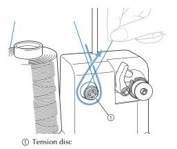
Pass the thread through the hole in the right 5 of the thread guide toward the back of the machine.
