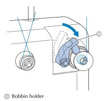
Press the main power switch to start winding the bobbin.
