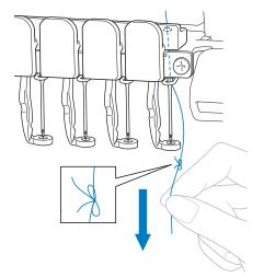
Continue pulling the thread until the knot is above the needle. Cut the knot.
