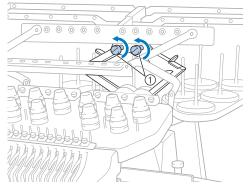
Turn the screw counterclockwise three or four times to loosen it.
