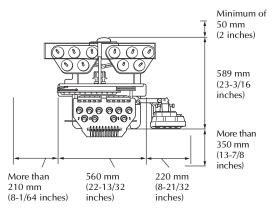
Adjust the legs so that the machine is steady. Use the included wrench to loosen the lock nut on the leg that you wish to adjust.
