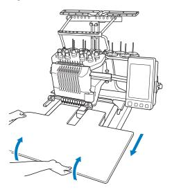
After the pins on each side reach the notches 2 in the guide plates, raise the table to lift the pins up through the notches.
