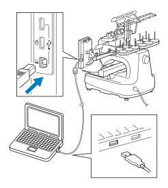
If the machine is positioned at a distance that prevents the USB cable from reaching the computer, embroidery patterns can be transferred from the computer by temporarily saving them on USB media, which is then connected to the machine. (Refer to "USB media" on page 173.)
