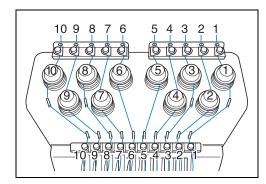
Pass the thread through the hole in the number 1 upper thread guide and pull the thread toward you.
