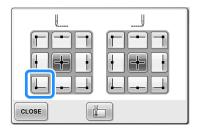
The frame moves so that the needle drop point aligns with the beginning of stitching.
