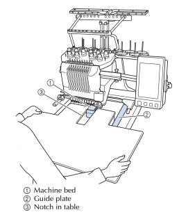
**3** Pull the table toward you until the pins on the mounting brackets (attached on each side to the bottom of the table) fit into the notches in the guide plates.
