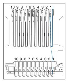
8 Pass the thread along the number 1 slot to pass it through the number 1 take-up lever hole from right to left.
