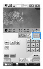
Touch the positioning keys to move the embroidery frame until the thread mark on the fabric is aligned on the starting point in the camera view window.
