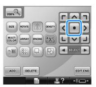
The pattern can also be moved by dragging it. If a USB mouse is connected, move the mouse to position the pointer on the desired pattern, and then hold in the left mouse button while dragging the pattern. The pattern can also be dragged by selecting it directly in the screen with your finger or the touch pen.
