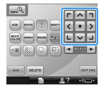
► The pattern moves in the direction of the arrow on the key.
