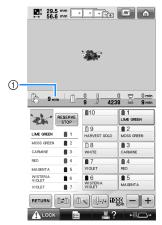
① Time until the machine stops
