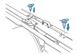
While pushing in the cap frame driver toward the machine so that it is fully inserted, tighten the two lower thumb screws to secure the cap frame driver.
