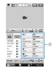
① The threads threaded on the needle bars are indicated as shown here.
