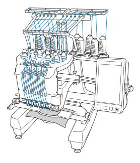
Not all ten needles can be used to sew at the same time. Only one needle is moved to the embroidering position at a time. According to the sewing order, the needle bar case is moved to the left and right so that the needle bar and needle thread with the required color can be moved to the embroidering position.
