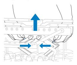
After the thread guide assembly support is extended and the thread guide assembly is raised to its highest position, tighten the two thumb screws to secure the thread guide assembly in place.
