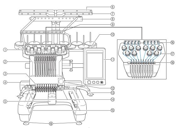
① Thread tension knobs
