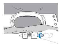
If the screw was tightened using a discshaped screwdriver, use the included discshaped screwdriver to loosen it.
