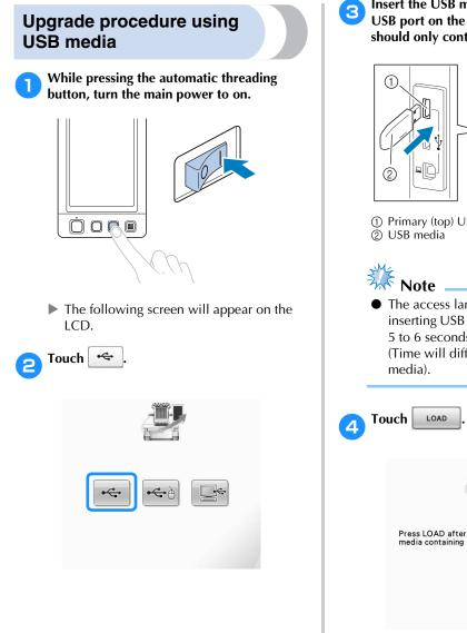
Insert the USB media into the primary (top) USB port on the machine. The media device should only contain the upgrade file.
