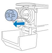
**3** Rotate the handwheel (about 50 degrees) to move the race of the hook to a position where it can easily be oiled.
