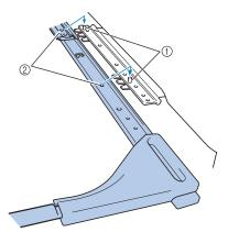
Pins in the frame-mounting plate
